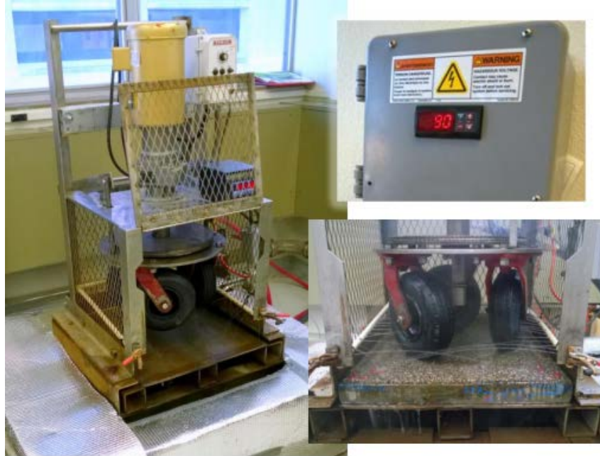
Figure 22. NCAT Three-Wheel Polisher with Water Bath.
